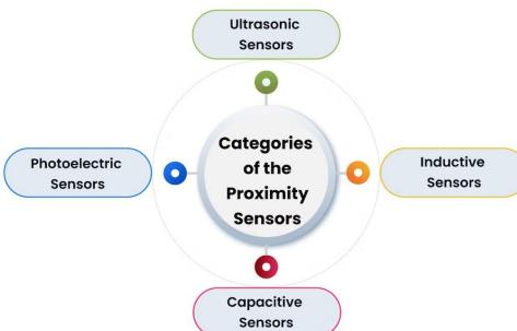
Proximity sensors detect the presence or absence of objects near the sensor without physical contact. They often emit a beam of radiation like infrared or an electromagnetic field. They can be used for process monitoring and control, object counting, assembly lines, and determining available space. Proximity sensors are common in retail settings, industrial complexes, and parking lots. Some examples are photoelectric, magnetic, capacitive, inductive, and ultrasonic.
