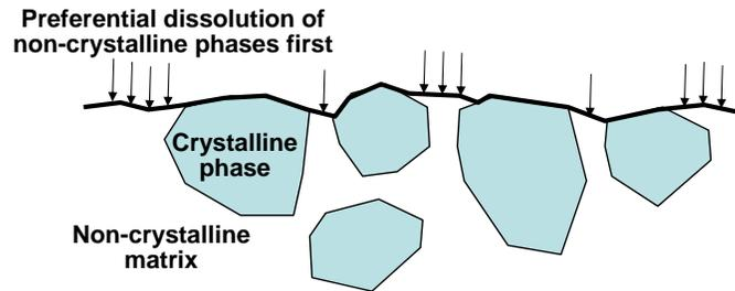
Ceramics rarely undergo anything comparable to metal chemical corrosion or electrochemical corrosion.
