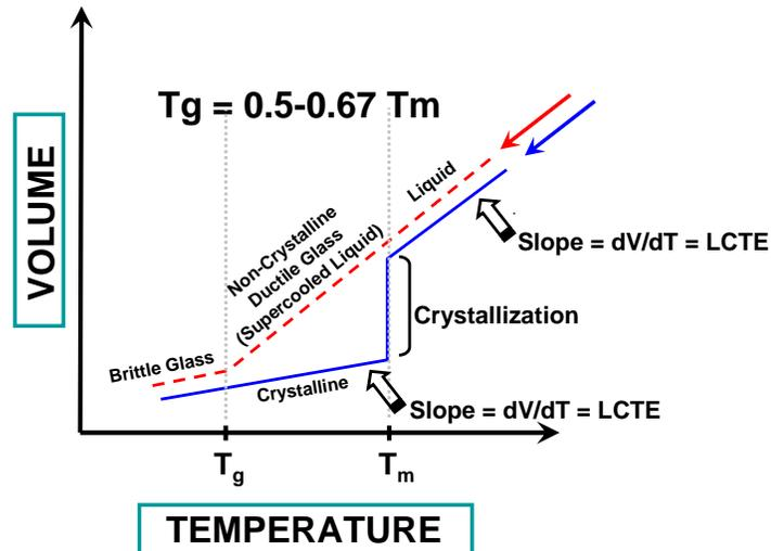
To understand this behavior you need to understand the GLASS TRANSITION temperature that is associated with the non-crystalline phase. Let's go through the diagram shown.
