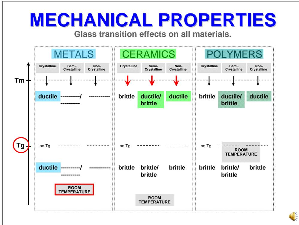
The glass transition temperature is relevant to any solid that contains non-crystalline material. Metals are difficult to keep from crystallizing but if quenched fast enough, they can exhibit non-crystalline phases. Ceramics are often semi-crystalline. Polymers are generally non-crystalline.
