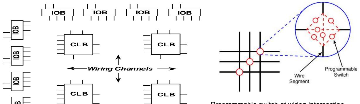
Programmable switch at wiring intersection (credit: www.wikipedia.com)
