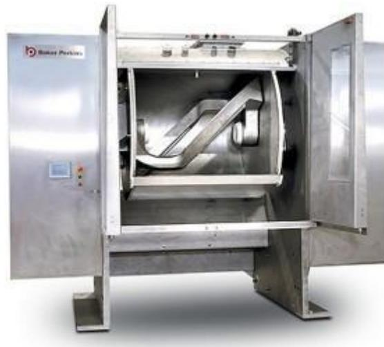
Some hard doughs are mixed to a pre-set temperature. The mixer blade provides a vigorous extruding and shearing action to develop the gluten web and this action results in an increase in temperature. The dough temperature is monitored by a thermocouple in the wall of the mixer bowl.
