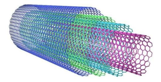
MWNTs have outer diameter in range of 2 - 100 nm depending on number of coaxial tubes present.
