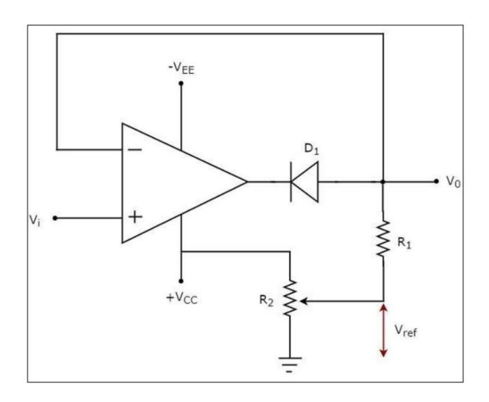
• The value of the reference voltage Vref can be chosen by varying the resistor R2.
