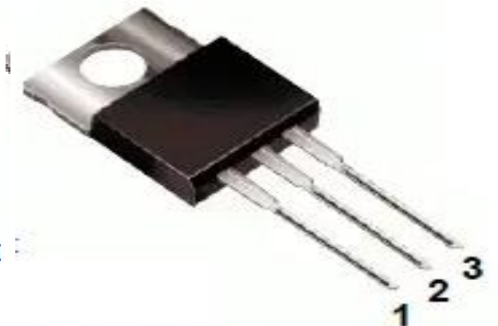
LM317 Pin Arrangement
