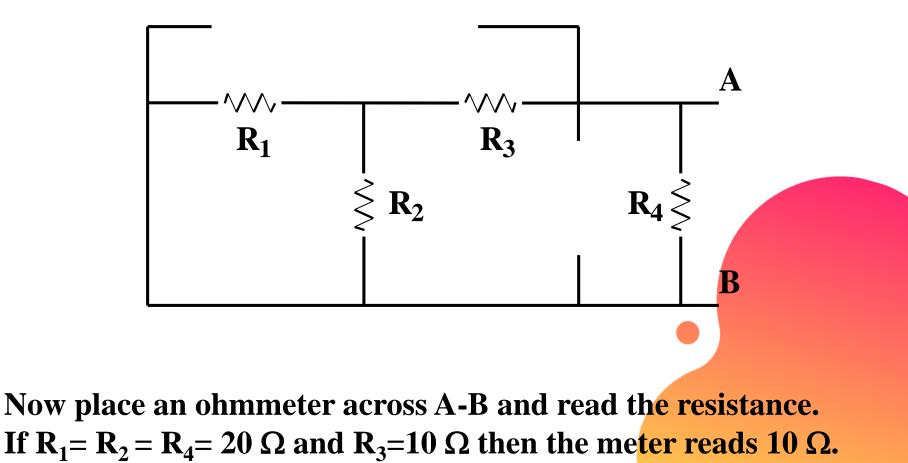
We call the ohmmeter reading, under these conditions,  $R_{THEVENIN}$  and shorten this to  $R_{TH}$ . Therefore, the important results are that we can replace Network 1 with the following network.
