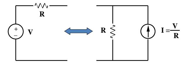
In view of the above, if we have the Thevenin equivalent circuit of a network, we can obtain the Norton equivalent by using source transformation.
