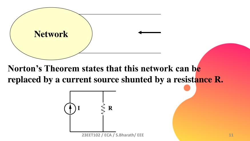
In the Norton circuit, the current source is the short circuit current of the network, that is, the current obtained by shorting the output of the network. The resistance is the resistance seen looking into the network with all sources deactivated. This is the same as  $R_{TH}$ .
