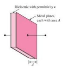
A capacitor consists of two conducting plates separated by an insulator (or dielectric).
