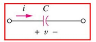
The current-voltage relationship of capacitor according to above convention is
