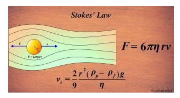
viscous drag force acting on a small sphere moving through a fluid under the influence of gravity.
