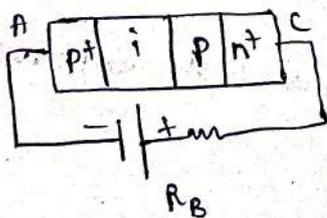
when the light is applied, light enters into p+ region to i region, the photons are interact with atoms in the intrinsic region.
