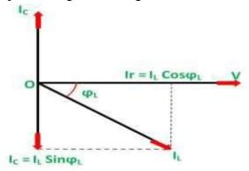
At the Resonance condition, the circuit draws the minimum current as under this (resonance) condition the reactive component of current is suppressed.
