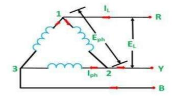
The current flowing through each phase is called **Phase Current (Iph)**, and the current flowing through each line conductor is called **Line Current (I<sub>L</sub>)**.
