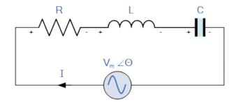
In a series RLC circuit there becomes a frequency point were the inductive reactance of the inductor becomes equal in value to the capacitive reactance of the capacitor. In other words,  $X_L = X_C$ . The point at which this occurs is called the Resonant Frequency point, ( $f_r$ ) of the circuit, and as we are analyzing a series RLC circuit this resonance frequency produces a Series Resonance.
