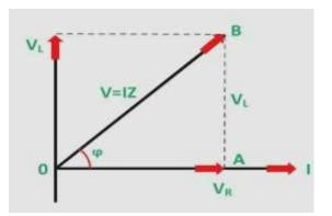
Steps to draw the Phasor Diagram of RL Series Circuit
