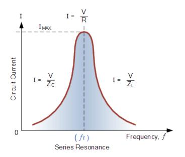
The frequency response curve of a series resonance circuit shows that the magnitude of the current is a function of frequency and plotting this onto a graph shows us that the response starts at near to zero, reaches maximum value at the resonance frequency when  $I_{MAX} = I_R$  and then drops again to nearly zero as *f* becomes infinite. The result of this is that the magnitudes of the voltages across the inductor, L and the capacitor, C can become many times larger than the
