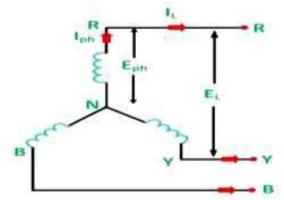
Considering the above figure, the finish terminals of the three windings are connected to form a star or neutral point. The three conductors named as R, Y and B run from the remaining three free terminals as shown in the above figure.
