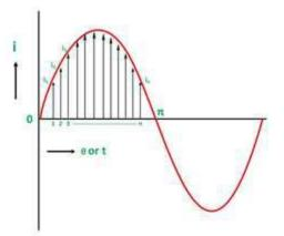
Divide the positive half cycle into (n) number of equal parts as shown in the above figure
