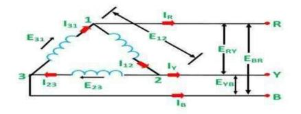
It is clear from the figure that the voltage across terminals 1 and 2 is the same as across the terminals R and Y. Therefore,
