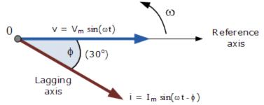
The phasor diagram is drawn corresponding to time zero (t = 0) on the horizontal axis. The lengths of the phasors are proportional to the values of the voltage, (V) and the current, (I) at the instant in time that the phasor diagram is drawn. The current phasor lags the voltage phasor by the angle,  $\Phi$ , as the two phasors rotate in an *anticlockwise* direction, therefore the angle,  $\Phi$  is also measured in the same anticlockwise direction.
