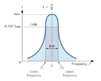
The frequency response of the circuit's current magnitude above, relates to the "sharpness" of the resonance in a series resonance circuit. The sharpness of the peak is measured quantitatively
