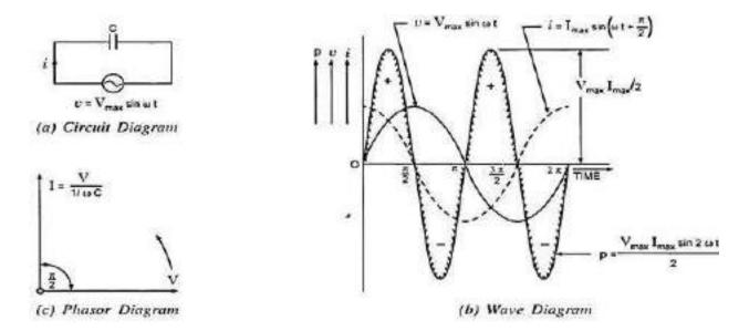
et an alternating voltage represented by  $v = V_{max} \sin \omega t$  be applied across a capacitor of capacitance C farads.
