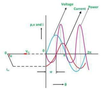
The various points on the power curve are obtained by the product of voltage and current. If you analyze the curve carefully, it is seen that the power is negative between angle 0 and  $\phi$  and between 180 degrees and (180 +  $\phi$ ) and during the rest of the cycle the power is positive. The current lags the voltage and thus they are not in phase with each other.
