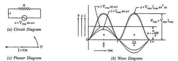
When the current flowing through a pure resistance changes, no back emf is set up, therefore, applied voltage has to overcome the ohmic drop of iR only
