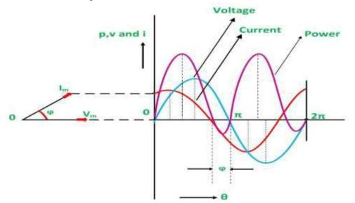
The various points on the power curve are obtained from the product of the instantaneous value of voltage and current.
