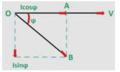
Taking voltage V as reference, the current I lags behind the voltage V by an angle  $\phi$ . The current I is divided into two components:
