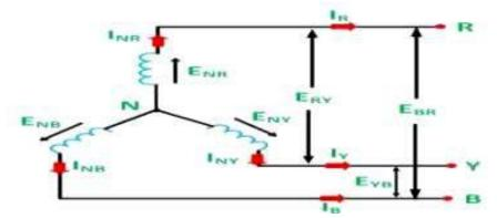
As the system is balanced, a balanced system means that in all the three phases, i.e., R, Y and B, the equal amount of current flows through them. Therefore, the three voltages  $E_{NR}$ ,  $E_{NY}$  and  $E_{NB}$  are equal in magnitude but displaced from one another by 120 degrees electrical.
