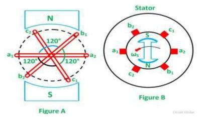
Consider three identical coils  $a_1a_2$ ,  $b_1b_2$  and  $c_1c_2$  as shown in the above figure. In this figure  $a_1$ ,  $b_1$  and  $c_1$  are the starting terminals, whereas  $a_2$ ,  $b_2$  and  $c_2$  are the finish terminals of the three coils. The phase difference of 120 degrees has to be maintained between the starts terminals  $a_1$ ,  $b_1$  and  $c_1$ .
