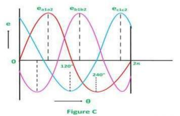
Considering the figure C, the analysis about their magnitudes and directions are given as follows. The emf induced in the coil  $a_1a_2$  is zero and is increasing in the positive direction as shown by the waveform in the above figure C represented as  $e_{a_1a_2}$ .
