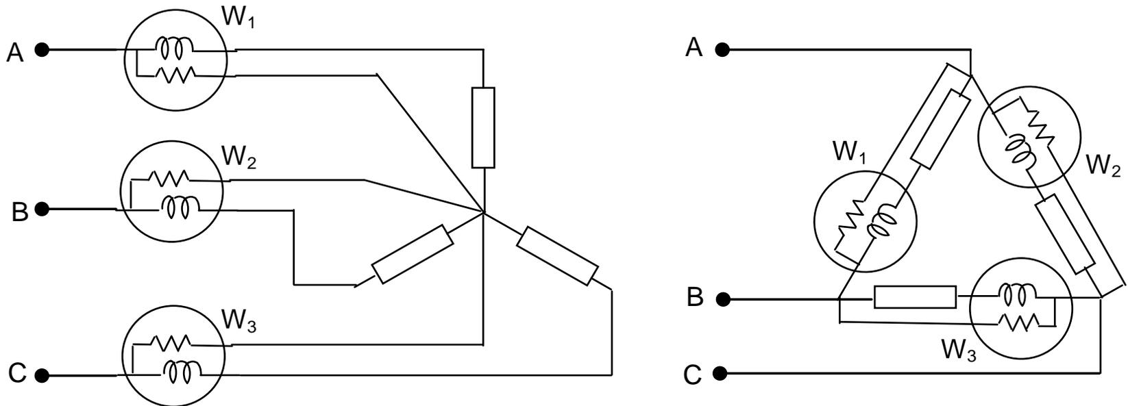
Fig. 6.27 Power measurement - Three wattmeters.
