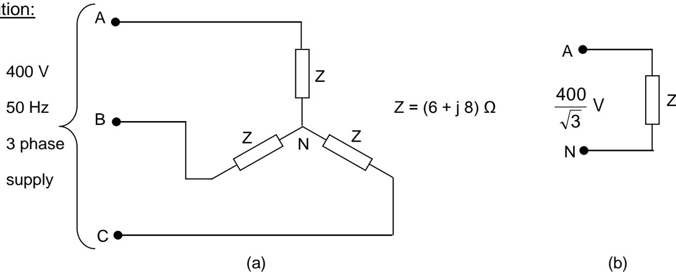
Given three-phase circuit and its **single-phase equivalent** are shown above. Referring to Fig. (b), Voltage  $E_{ph} = 400 / \sqrt{3} = 230.94 \text{ V}$ ;  $Z = (6 + j 8) \Omega = 10 \angle 53.13^\circ \Omega$
