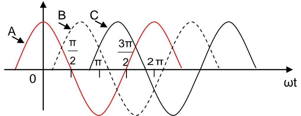
Because of the symmetry, these voltages are known as balanced three-phase voltages. The phasor descriptions of these three voltages are shown in Fig. 6.1 in which voltage  $E_{AA'}$  is taken as reference.
