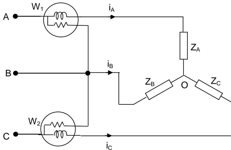
Fig. 6.32 Two wattmeter method - Star-connected unbalanced load.
