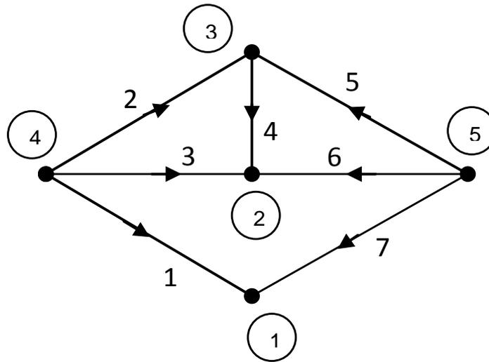
Fig. 9.17 Oriented graph with element and node numbers.
