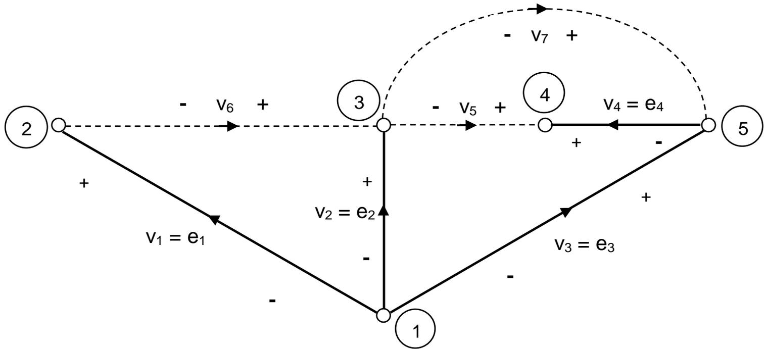
Further, using KVL, other element voltages can be obtained in terms of the tree branch voltages as given below.
