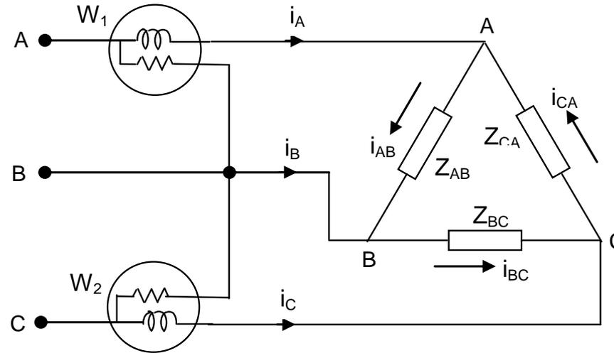
Fig. 6.33 Two wattmeter method - Delta-connected unbalanced load.
