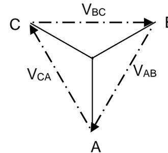
Fig. 6.11 Phasor diagrams - Phase sequence ACB.
