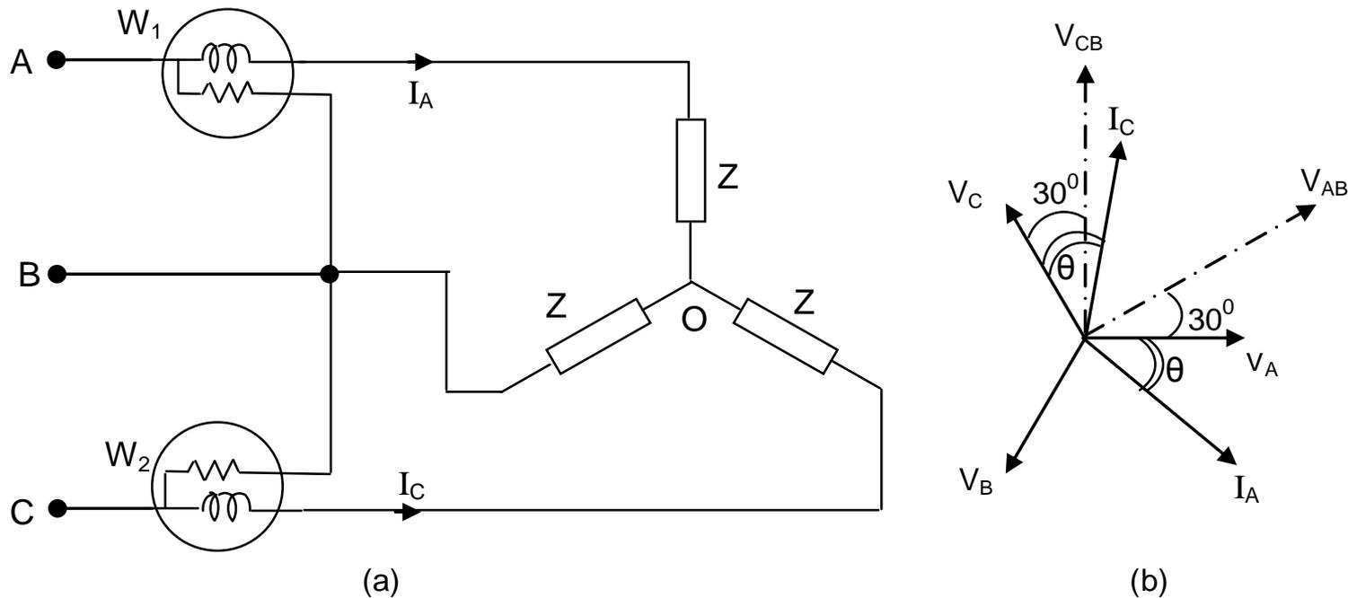
Fig. 6.28 Two wattmeter method - Star-connected balanced load.
