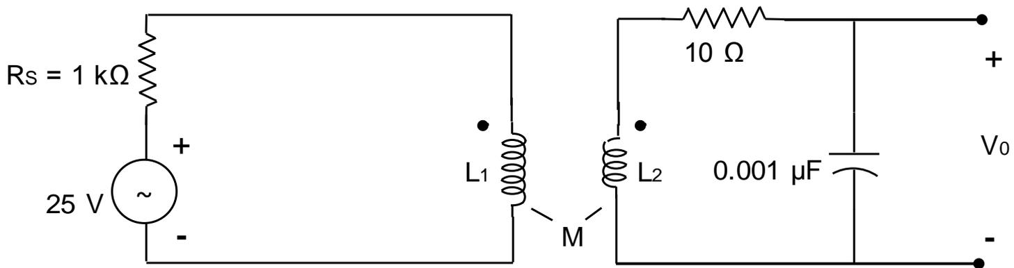
Fig. 4.92 Circuit for Example 4.47
