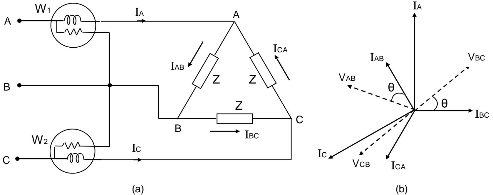
Fig. 6.29 Two wattmeter method - Delta-connected balanced load.
