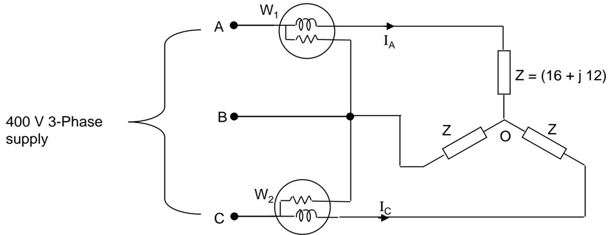
(a)  $V_A = \frac{400}{\sqrt{3}} \angle 0^\circ = 230.9410 \angle 0^\circ \text{ V}; \quad Z = (16 + j12) = 20 \angle 36.87^\circ \Omega$
