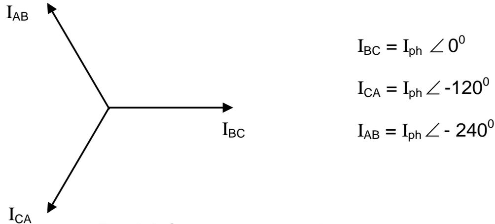
Fig. 6.6 Current phasors of phase currents in a delta system.
