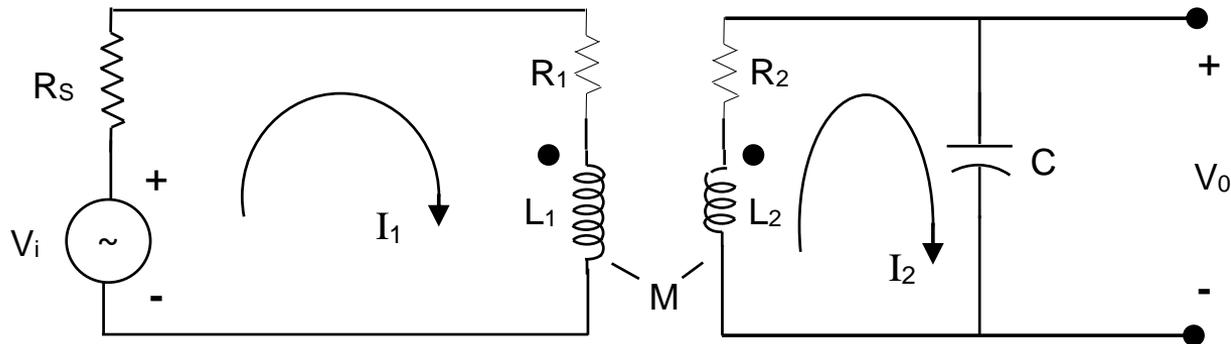
Fig. 4.91 Single tuned circuit.
