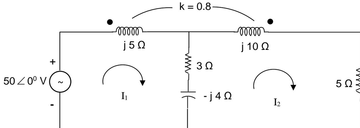
$$M = k\sqrt{L_1 L_2}; \text{ Multiplying by } \omega, X_m = k\sqrt{X_{L1} X_{L2}} = j 0.8\sqrt{5 \times 10} = j 5.65685 \Omega$$
