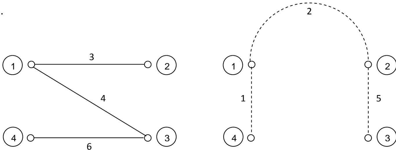
Fig. 9.5 A tree and the corresponding co-tree of a network graph.
