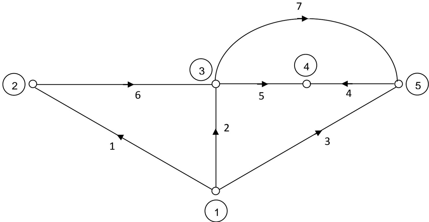
Fig. 9.13 Oriented connected graph.
