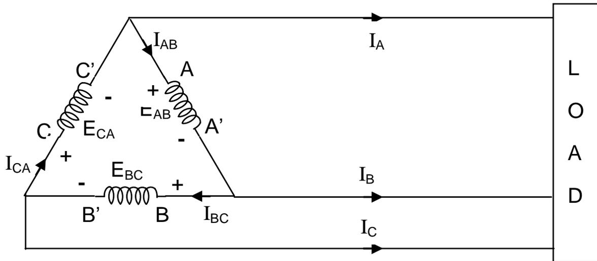
Line voltage,  $E_l =$  Phase voltage,  $E_{ph}$
