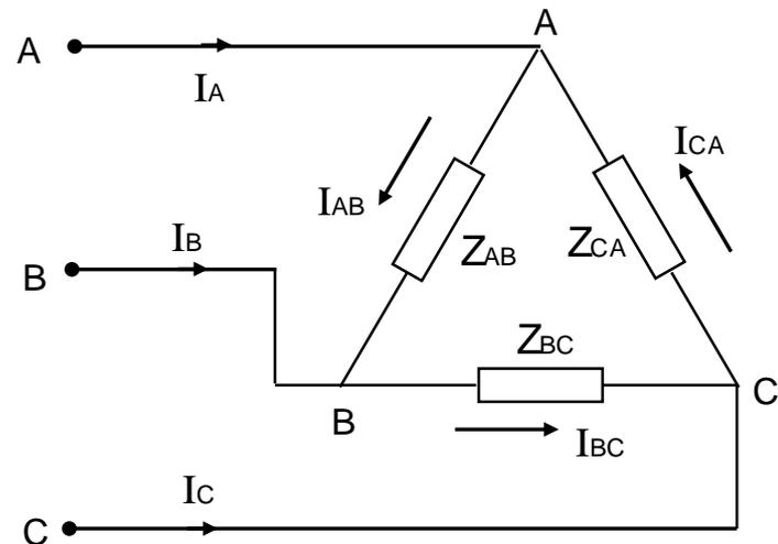
$$V_{BC} = 240 \angle 0^\circ \text{ V}; V_{CA} = 240 \angle -120^\circ \text{ V}; V_{AB} = 240 \angle -240^\circ \text{ V};$$
