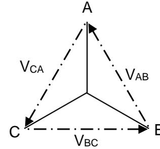
Fig. 6.10 Phasor diagrams - Phase sequence ABC.
