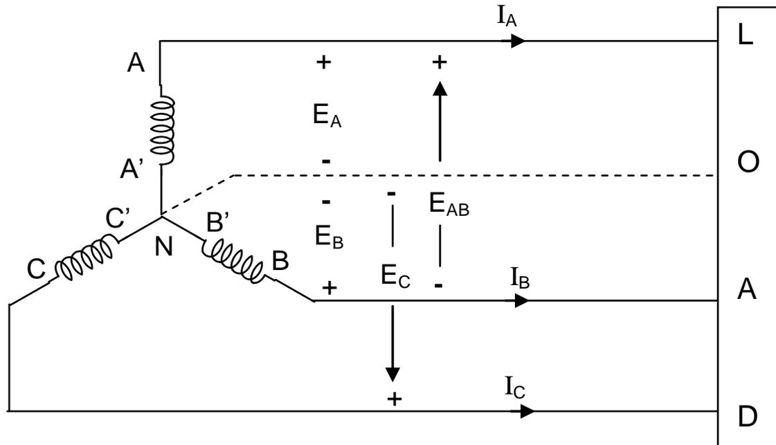
Let  $I_\ell$  and  $I_{ph}$  be the magnitude of line and phase currents and  $E_\ell$  and  $E_{ph}$  be the magnitude of line and phase voltages. In the case of star-connected three-phase system, as seen from Fig. 6.2, line current is equal to the phase current, i.e.
