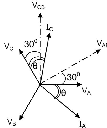
The phasor diagram, taking voltage  $V_A$  as reference is shown in Fig. 6.28 (b). The phasors  $V_{AB}$ ,  $V_{CB}$ ,  $I_A$  and  $I_C$  are indicated. Thus,
