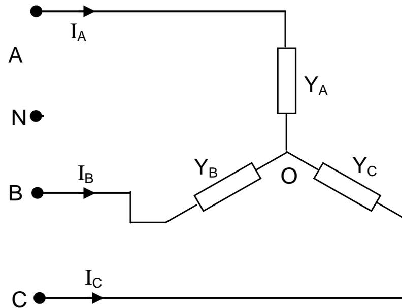
Applying KCL at point O we get  $I_A + I_B + I_C = 0$  i.e. (6.16)
