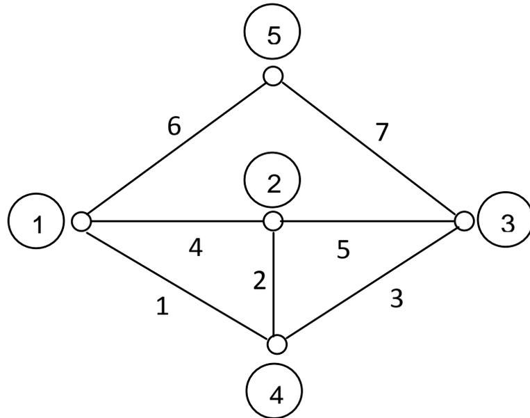
If the elements in a graph are assigned orientations, the resulting graph is called **ORIENTED GRAPH**. Fig. 9.3 shows an oriented graph.
