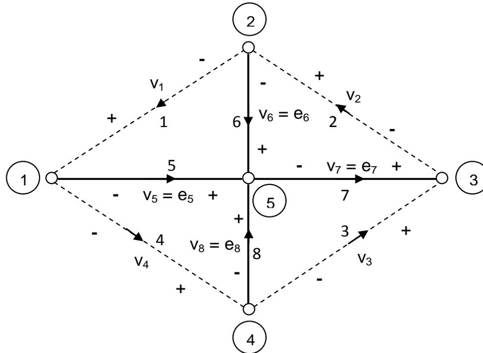
Fig. 10.21 Element and tree branch voltages - Example 10.2.
