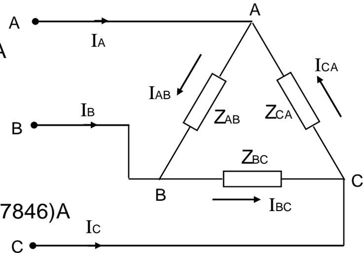
Line currents are obtained by applying KCL at junction A, B and C. Thus
