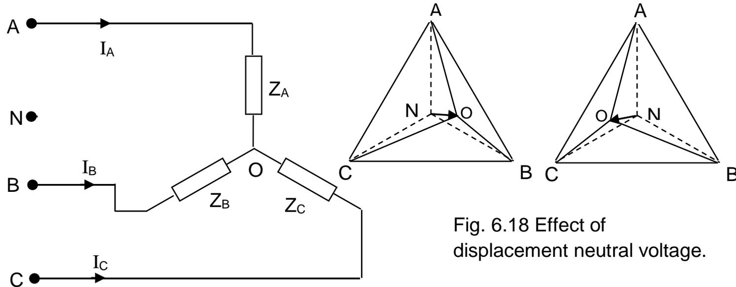
Fig. 6.18 Effect of displacement neutral voltage.
