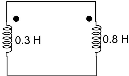
Fig. 4.82 Mutually coupled coils for Example 4.42.
