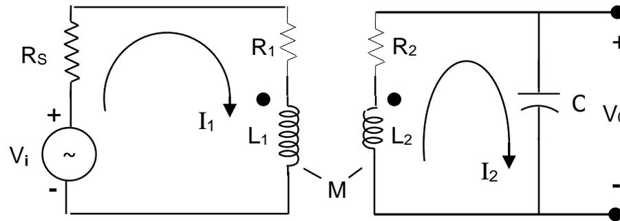
$$R_s I_1 - j \omega M I_2 = V_i \quad (4.188)$$
