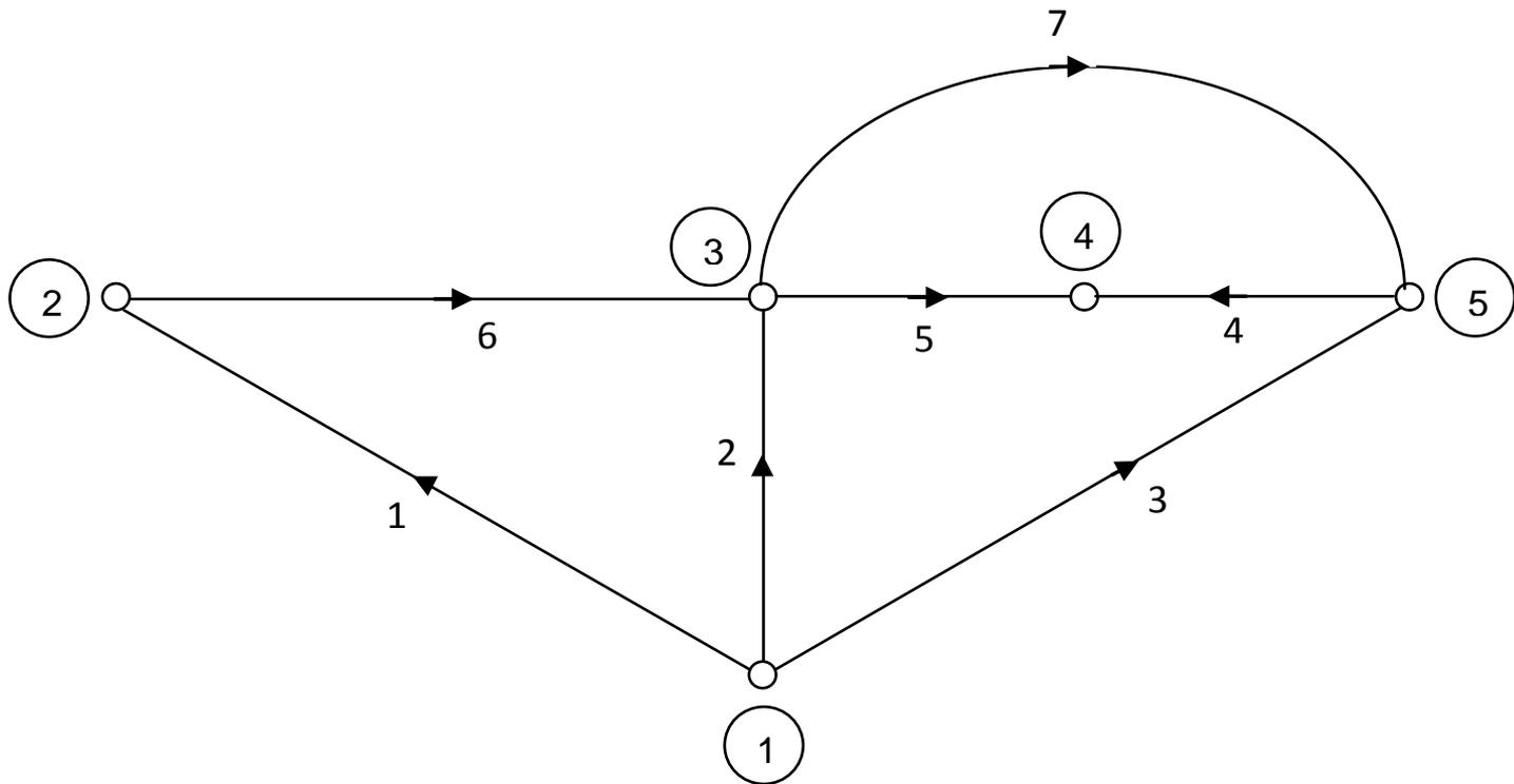
Fig. 9.8 Oriented connected graph.
