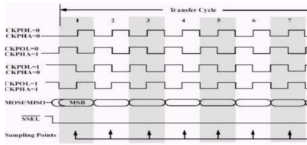
Timing Diagram – Showing Clock polarities and phases http://www.maxim-ic.com.cn/images/appnotes/3078/3078Fig02.gif
