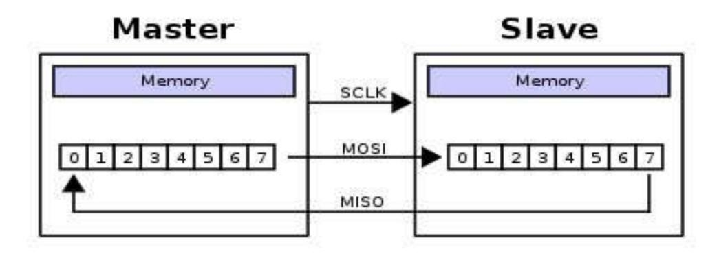
Master shifts out data to Slave, and shift in data from Slave http://upload.wikimedia.org/wikipedia/commons/thumb/b/bb/SPI\_8bit\_circular\_transfer.svg/400px-SPI\_8-bit\_circular\_transfer.svg.png
