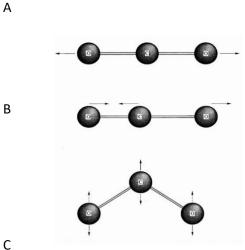
Symmetric stretching (a): In this mode, carbon atom remains stationery when the oxygen atoms oscillate simultaneously along the molecular. In this state CO<sub>2</sub> molecule will have energy that is intermediate as compared to that in the other two modes of vibrations (b and C). This state is referred in the spectroscopy as 100 state.
