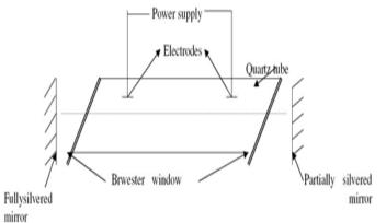
incident light whereas the other one is partially silvered to get polarized laser beam output.
