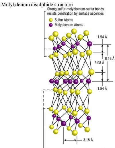
Weak sulfur-sulfur bonds allow easy sliding of these layers resulting in low friction
