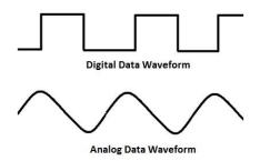
The main function of the modem is to convert digital signal into analog and vice versa. Modem is a combination of two devices — **modulator** and **demodulator**. The **modulator** converts digital data into analog data when the data is being sent by the computer. The **demodulator** converts analog data signals into digital data when it is being received by the computer.
