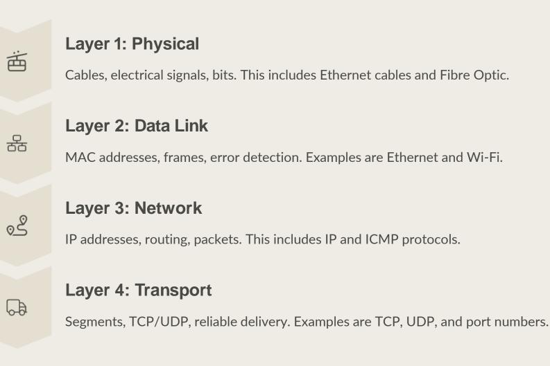
These lower layers are crucial for the physical transmission and initial handling of data. They manage addressing, routing, and reliable delivery across the network.
